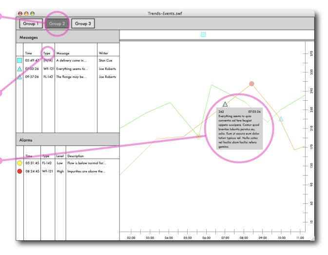
In this prototype, messages are integrated into the operator control screen as "stickies," which can be attached to components. The hope is that this will help facilitate Monitor to Monitor communication, as well as enhance situation awareness.
