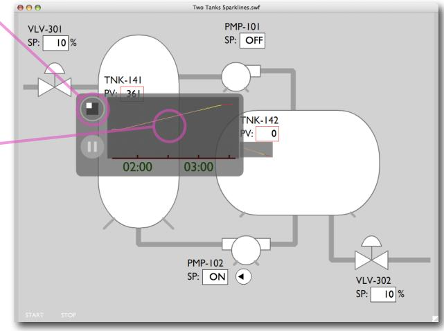
This is a prototype of a full-screen trends display which features the ability to display user-created messages which have been attached to particular trends or components. This fulfills the need for a fullscreen consolidated view of alarms and messages.
